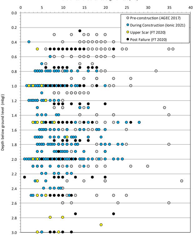
Undrained Vane Shear Strength of Peat (kPa)
