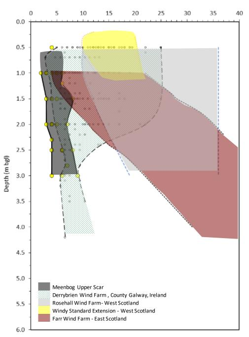
Undrained Shear Strength from Insitu Vane, cu (kPa)
